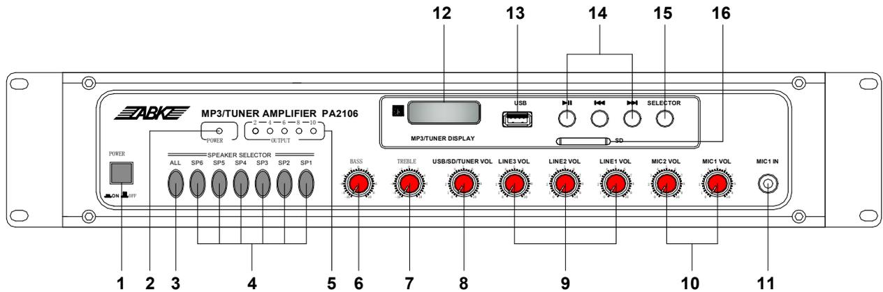
1. Power switch (power indicator lighting as ON state) for main power.
